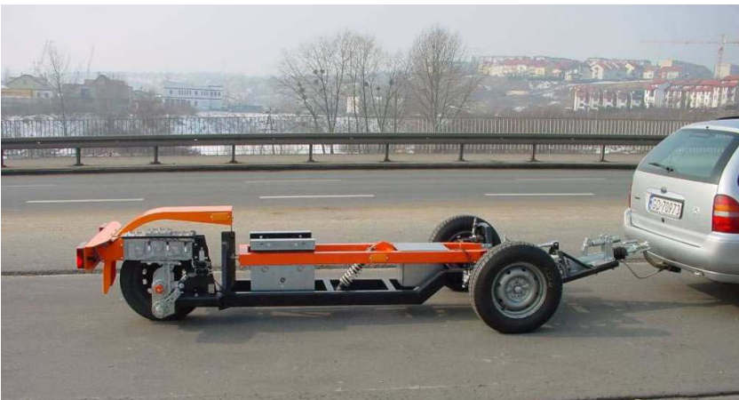
Rolling resistance measurement using measuring trailer from TU Gdansk
